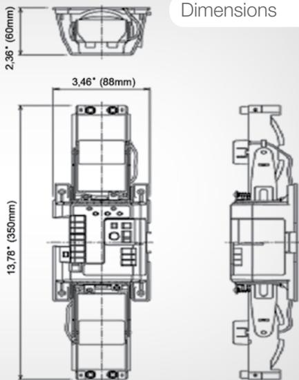
Available to cover up to 200m, this infrared beam feature a unique Double Modulated Beam signal making them extremely resistant to both direct and reflected sunlight up to 50,000 lux.
